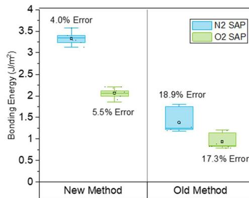
Fig 1. Bonding Energy of Fusion Bonded SiO<sub>2</sub> Wafers Treated by a N<sub>2</sub> or O<sub>2</sub> SAP.
